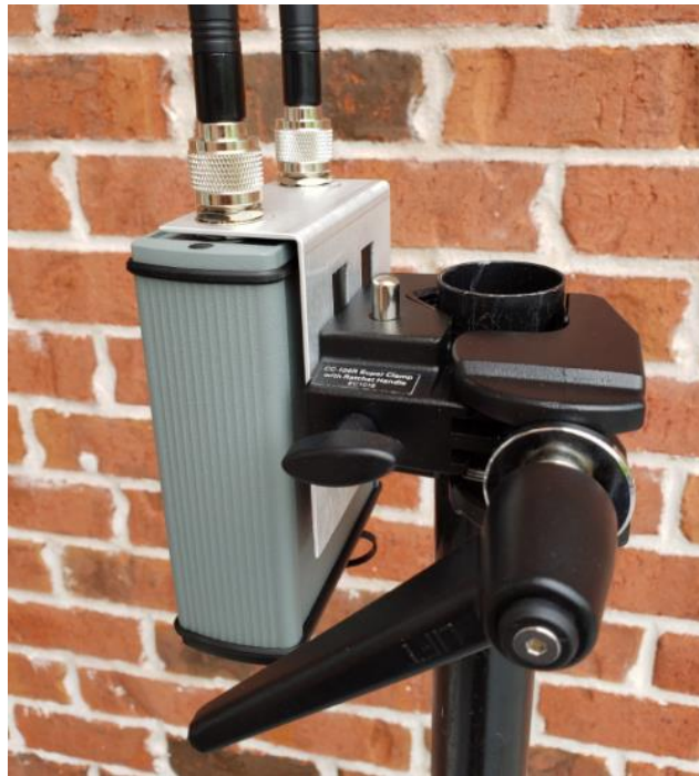
Figure 13 - STARX L-Mount shown with customer-provided Manfrotto SuperClamp
