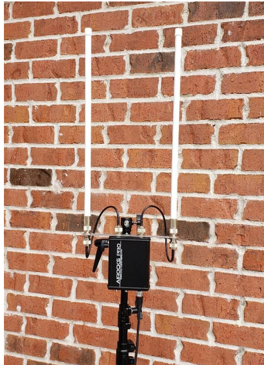
Figure 8 ARX-1900 with Dual 5db Omni Antennas
