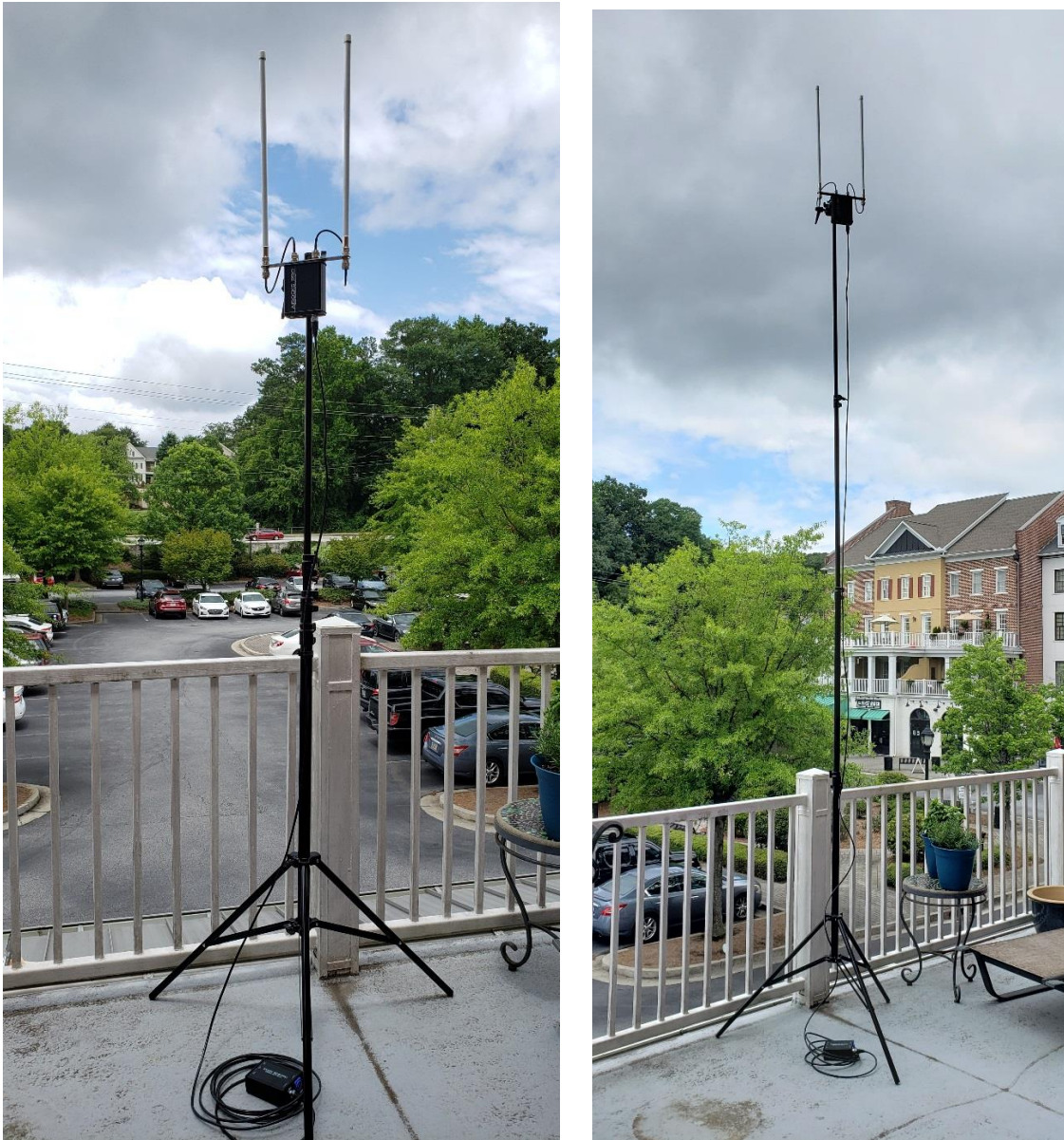
Figure 7 ARX-1900 on Flashpoint 13' Air Cushioned Heavy Duty Light Stand
